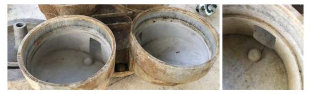
We inspected the Top Clovers and found that the inner sealing surfaces were rough which would not aid the o'rings to form a perfect seal. Some were showing cracks that would cause leakage. The Clovers (Top & Bottom) will need to be replaced.
