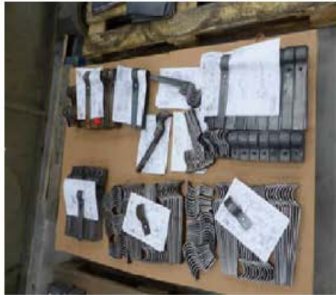
Steam Turbine Generator – Fabricating pipeline hangers
