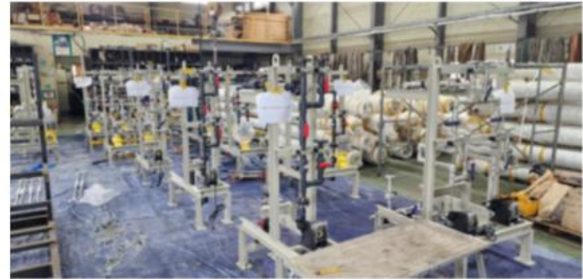
Waste Water Treatment System – Manufactured Chemical Dosing Skid
