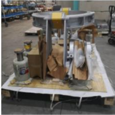
Steam Turbine Generator – Packing piping supports for shipping
