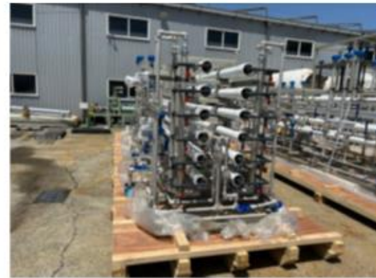
Waste Water Treatment System – Packing RO unit for shipping
