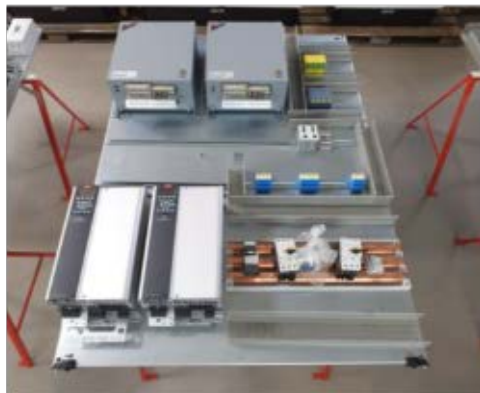
Fuel Oil Treatment System – Switch gear production in progress
