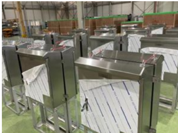
Local box - enclosure production completed
