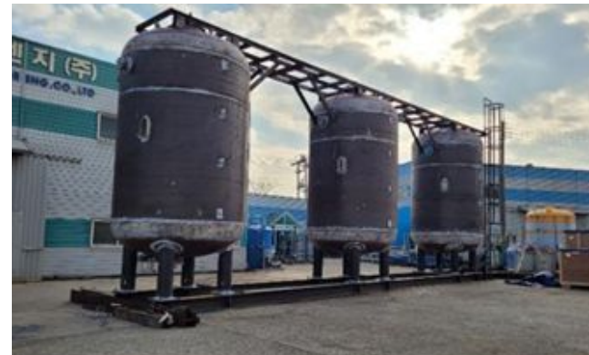
Water/Waster Water Treatment System – pressure vessel structure manufacturing in progress
