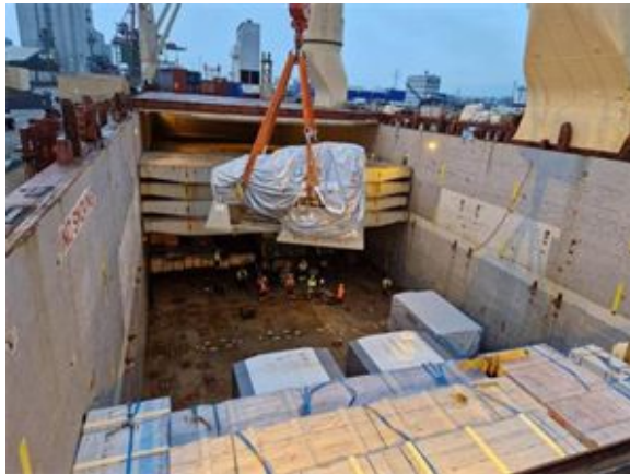
Steam Turbine and generator loaded into vessel
