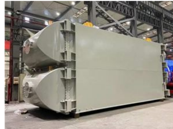
STG – condenser manufacturing in progress
